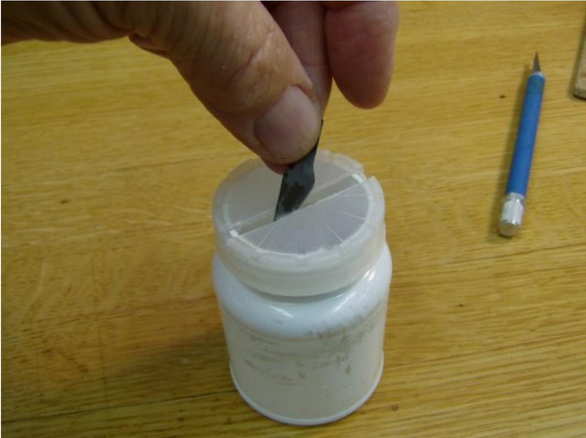
When I'm building or MonoKoteing a model I run thru a lot of X-acto blades. A good safe way to discard used blades is in a pill bottle with a slot cut in the top. When it's filled simply put a piece of masking tape over the slot and dispose in the trash.
